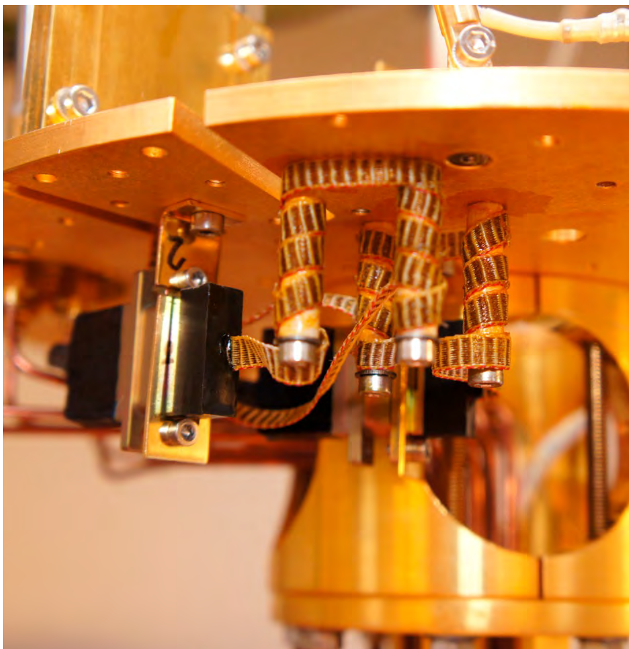
Inside stages of a dry dilution refrigerator (Oxford Instruments Triton 200). Photo: Adam Burke
