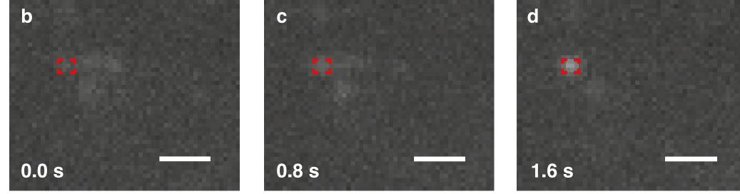
**Light guiding schematic and results.** a) Filaments can be transported horizontally above, vertically along nanowires and on the substrate. Light emitted from excited fluorophores on the filaments running vertically along wires is collectively emitted from the tips of the wires. b–d) Fluorescence micrographs of filament moving down a single wire (red dashed line). Scale bars: 2 µm.
